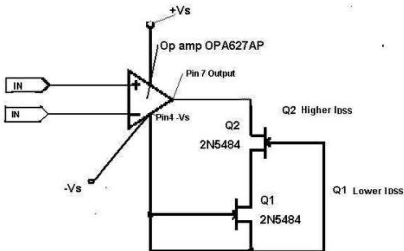
I need six PCBs that can hold two TO92 NPN Transistors in this configuration with the two output pins thin enough to slide next to the op amp pins (pins 4 & 7) through the main PCB. The two output pins need to be long enough for this device to stand over, straddling the op amp. Longer is better than shorter. This needs to be resistant to soldering the two transistors (63/37 RMA solder) and then to the main PCB without falling apart.
