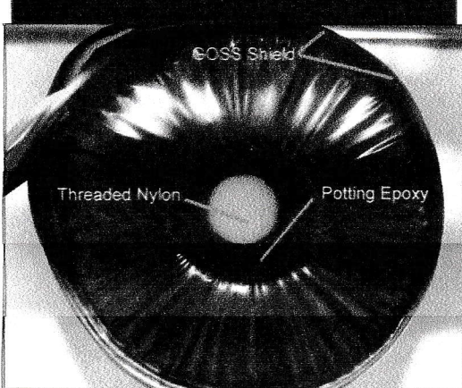
PHOTO 19: Plitron transformer after potting.
