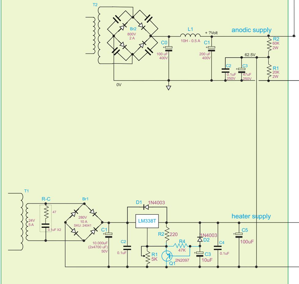
ch 1a - secondary power supply board
