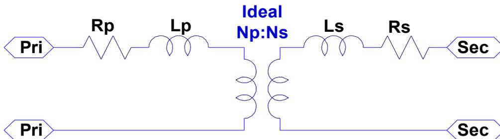
**Step 2:** The secondary and Ls are referred to the primary side as Rseq and Lseq.  $R_{seq} = R_s \times N_p / N_s$ ,  $L_{seq} = L_s \times N_p / N_s$ .
