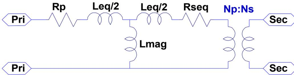
**Step 4:** Split the secondary into two equal parts.  $N_p/N_s$  is now half the previous. The values for  $R_{seq}$  and  $L_{seq}$  are not affected since they are on the primary side. So only secondary voltages and currents are changed. Each branch has  $R_{seq} \times 2$  since they are in parallel giving the net value of  $R_{seq}$  as previous. Likewise  $L_{seq}/2 \times 2$  for each branch which is shown as  $L_{seq}$  in the final model subcircuit above.
