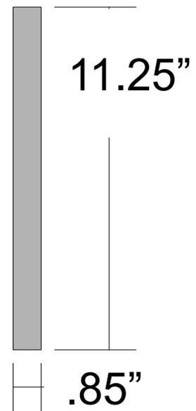
\* If using butt joints this should be 11.5" and not 13" also note that the top should rest on the top of the side pieces and repeat with the bottom this will make your cabinet the full 13" tall.
