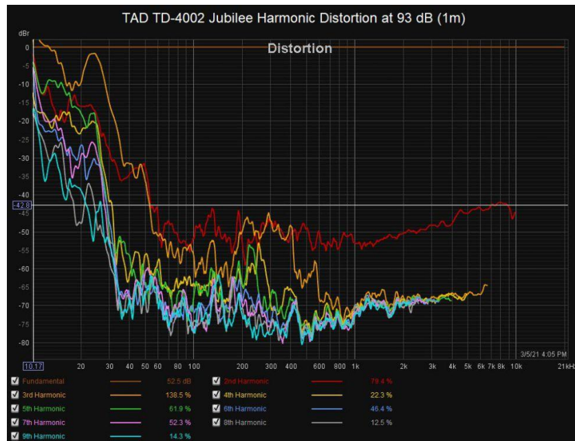
Figure 16 TAD TD-4002 harmonic distortion at 93 dB (1m) on K-402 horn
