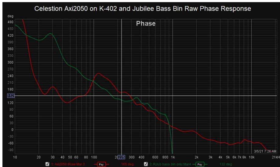
Figure 8 Phase response of first gen Jubilee bass bin and Celestion Axi2050 on K-402 horn
