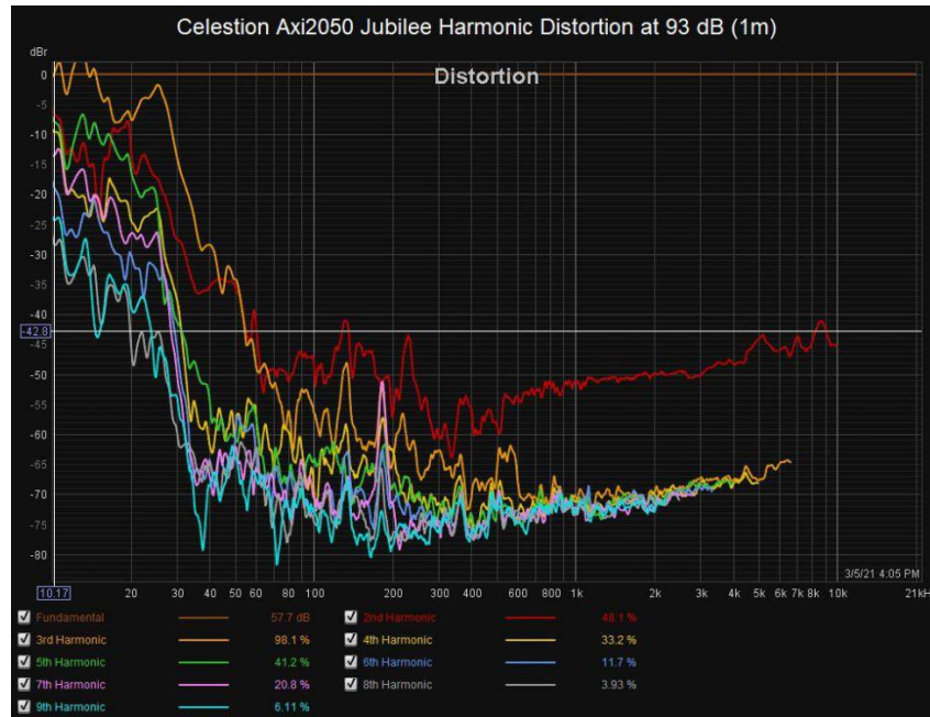
Figure 17 Celestion Axi2050 harmonic distortion at 93 dB (1m) on K-402 horn
