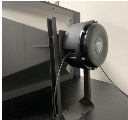
Figure 5 Celestion Axi2050 driver mounted on K-402 horn
