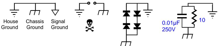
**Chassis Ground** Jumper J13 connects the PCB's ground to the chassis through the top leftmost mounting hole. If you wish to float the chassis or capacitor couple the chassis to ground, then either leave jumper J13 out or replace it with a small-valued capacitor ( $0.01$  to  $0.1\mu\text{F}$ ). Warning: if rubber O-rings are used with PCB standoffs, then the ground connection to the chassis is not likely to be made; in this case, use metal washer in place of top rubber O-ring.
