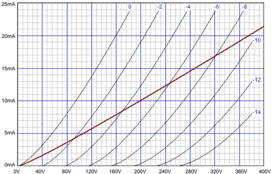
As the graph above reveals, a 6SN7 triode, with an unbypassed 430-ohm cathode resistor, behaves much like a 20k resistor. (By the way, note the much improved linearity over the plate curve traces, albeit at the cost of greatly increased plate resistance and reduced transconductance. Adding a plate resistor also makes the triode behave more like a good resistor.) The formula for the effective resistance (with an unbypassed cathode resistor) is:
