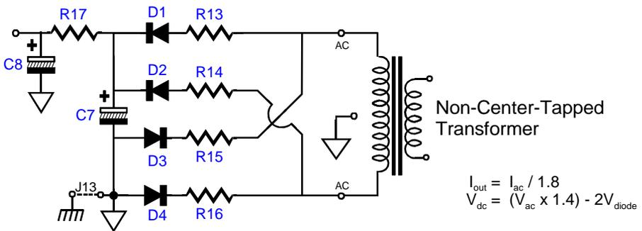
**Full-Wave Bridge** This is the most popular power supply configuration. The entire primary winding is used and four rectifiers are required. This configuration is seldom used with tube rectifiers, as the rectifier cathodes cannot be heated by just a single heater winding. The two solid-state diode voltage-drops count for little in a high-voltage power supply, but are a big liability in low-voltage power supplies.
