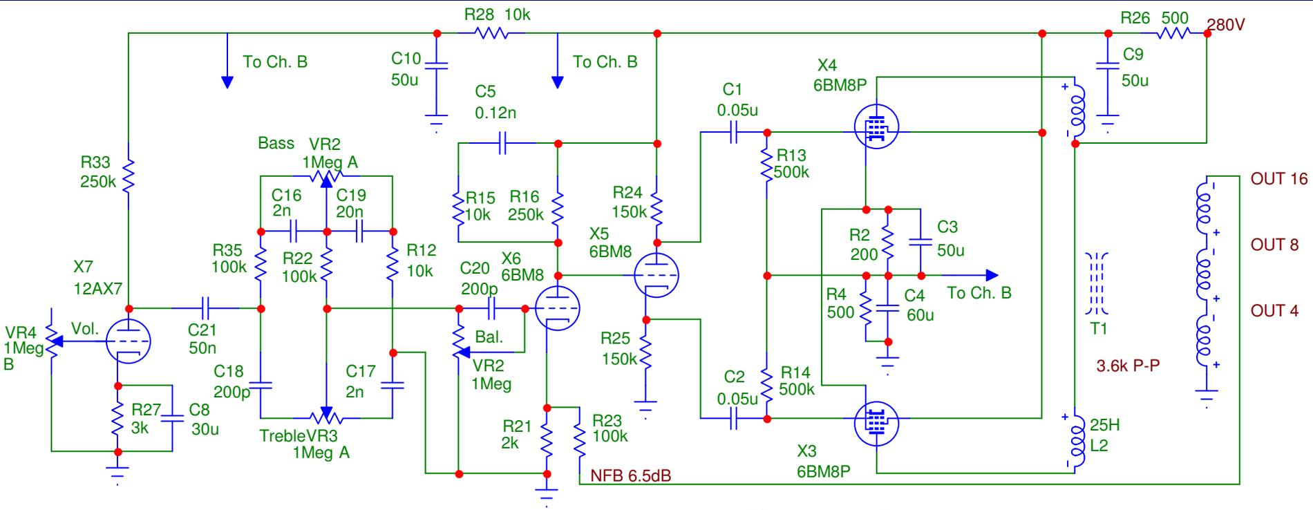
R4 is shared with Chb and is in parallel with two 12.6V heaters in series (combined R approx 126R)
