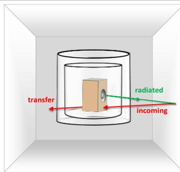
The Direct Sound Separation uses a double layer Scanning for identifying the direction of the sound waves. The Sound Field is fitted to a single sound source in the scanned surface and reflected sound passing through the scanned surface. Thereby radiated sound of the speaker is separated from reflected sound in the room (room modes). This powerful method allows a directivity measurement under non-anechoic conditions.
