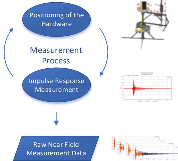
**Data Acquisition:** According to the required Setup, a grid of measurement points is calculated. The System automatically positions the hardware and runs a measurement of the Impulse response at every single point.
