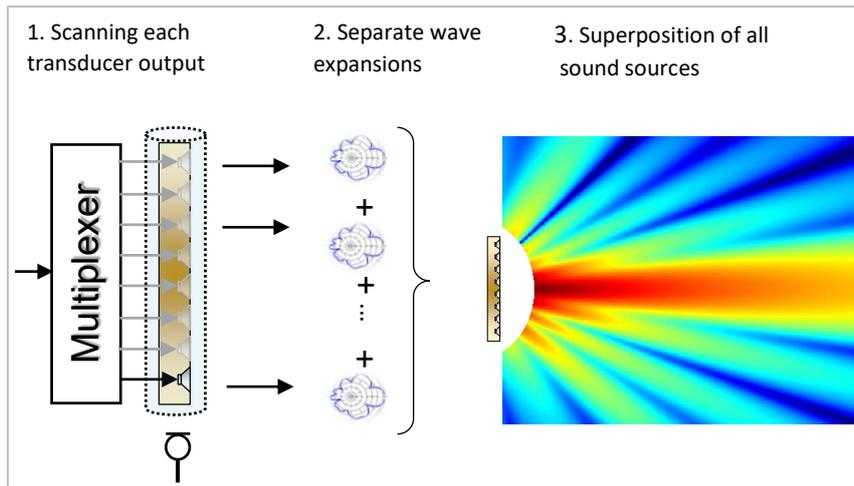
In addition to the analysis of the original sound field, the measured directivity data is an ideal basis for further simulation, because it includes acoustical effects (e.g. diffraction) of the loudspeaker cabinet as well.
