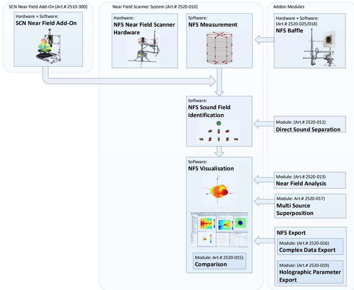
The Klippel Near Field Scanner is a measurement system, to measure the radiation characteristic of all sorts of sound sources. The principle of acoustic holography is used to combine the benefits of a near field measurement with the demand of the radiation characteristic in any distance. Based on the sound pressure measured in the very close near field, free field sound pressure is calculated at any distance.
