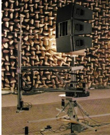
Line Array Segments are a very critical sound source to be measured in the near field. The critical characteristics are:
