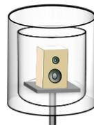
Scanning is done on two nested three dimensional cylindrical surfaces.
