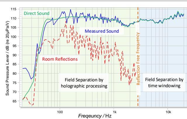
**Measured sound (blue):** Microphone signal measured in the near field. It is separated into radiated and transferred sound.
