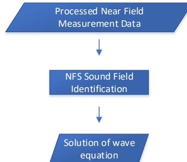
The sound field is identified as a weighted sum of spherical waves, which are built up by spherical harmonics  $Y_n^m(\theta, \phi)$  multiplied with Hankel functions  $h_n(kr)$  14.1, solving the wave equation.
