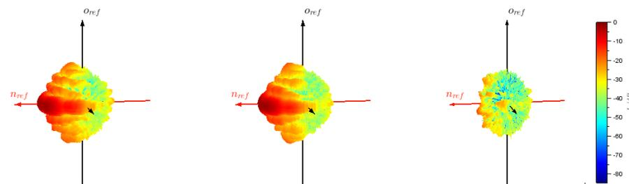
The measurements show a very little difference between NFS and Reference measurement. Especially in the most relevant main radiation direction the error is well below 20dB of the main lobes sound pressure
