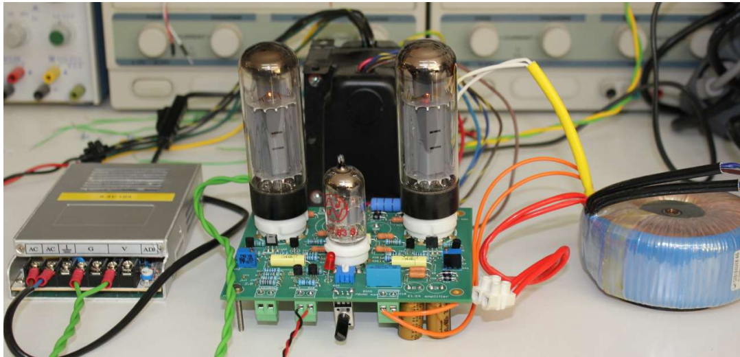
Photo of a finished amplifier channel with old EL34 tubes, a Hammond 1650N output transformer, impedance = 4,3 k ohms, power = 60 W and a 230 V AC / 6.3 V 10 A switching power supply (enough for two channel, recommended solution)
