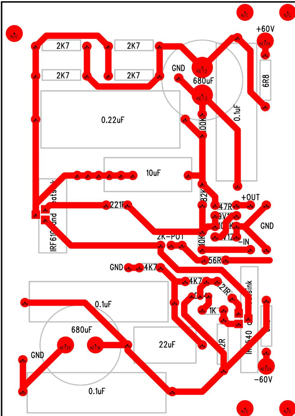
680uF caps are located on bottom side of PCB
