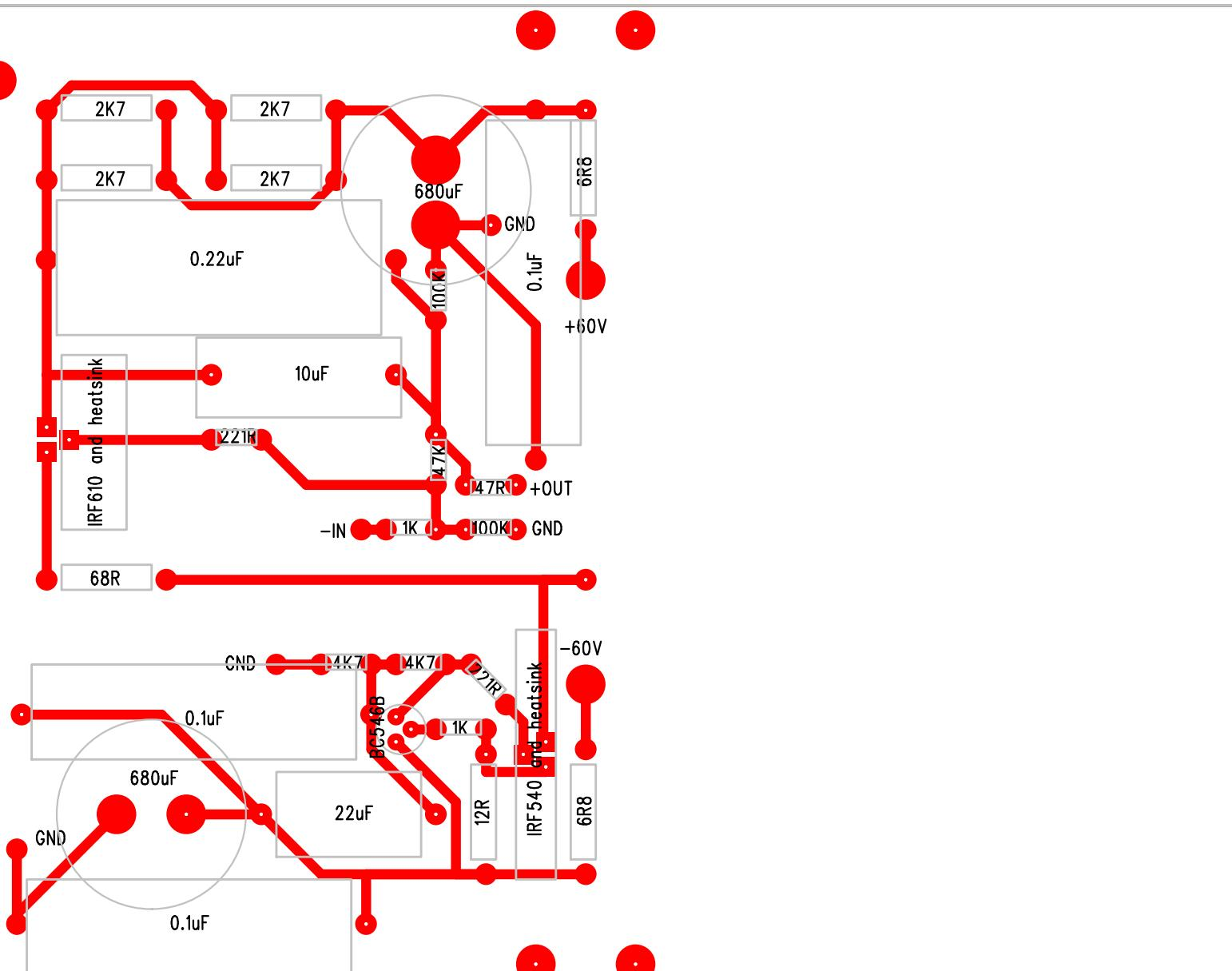
680uF caps are located on bottom side of PCB
