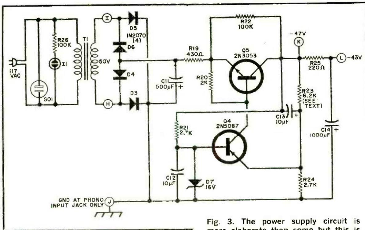
Fig. 3. The power supply circuit is more elaborate than some but this is essential to proper preamp operation.
