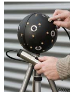
Fig. 5 36 channels spherical array with 12 cameras
