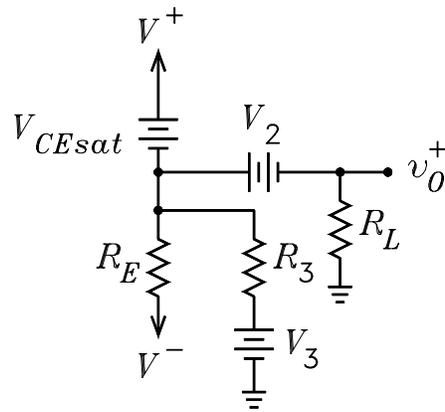
Figure 5: Circuit for calculating  $v_O^+$ .
