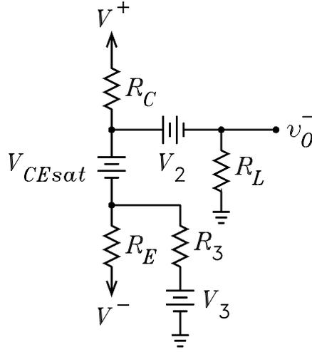
Figure 3: Circuit for calculating  $v_O^-$ .
