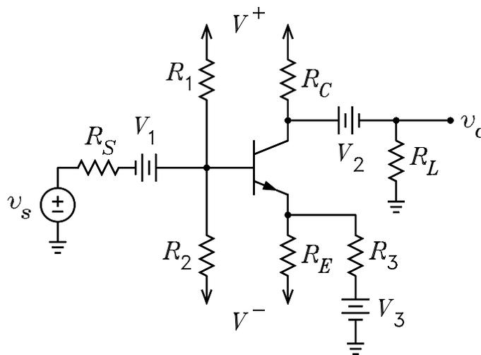
Figure 1: Common-emitter Amplifier.
