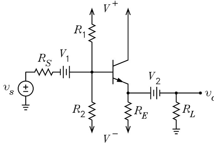
Figure 4: Common-collector amplifier.
