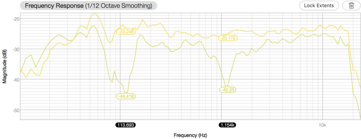
In Open Baffle designs I've always felt that having an OB woofer firing on both sides, but tweeter firing on only one side, never sounds quite right. So I added a SB Acoustics H250 horn and 44CD-T driver on the back. Photo:
