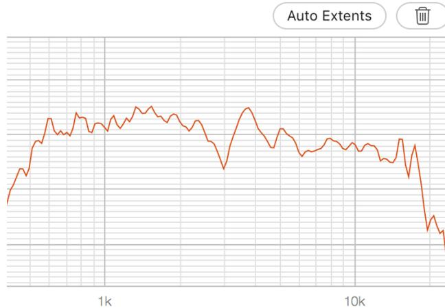
As you might expect, I EQ'd the tweeters with the MiniDSP and the Eclipse FIR software to obtain flat response both on and off axis.
