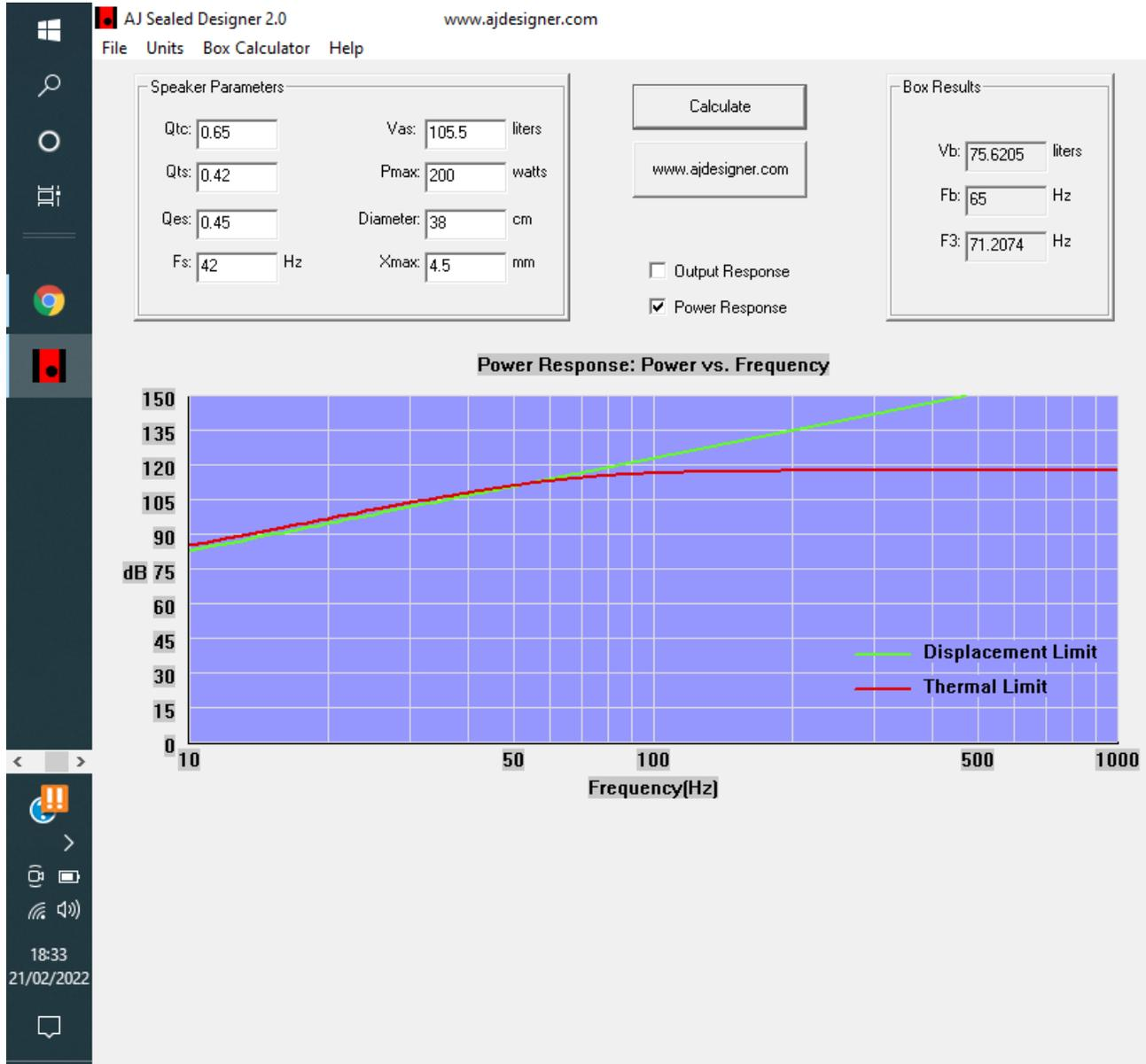
Beyma 15 inch 15LX60 V2 - Covering 40Hz to 300Hz- Sim with small sealed box (75 litres) @ 100% Xmax and 100% power.
