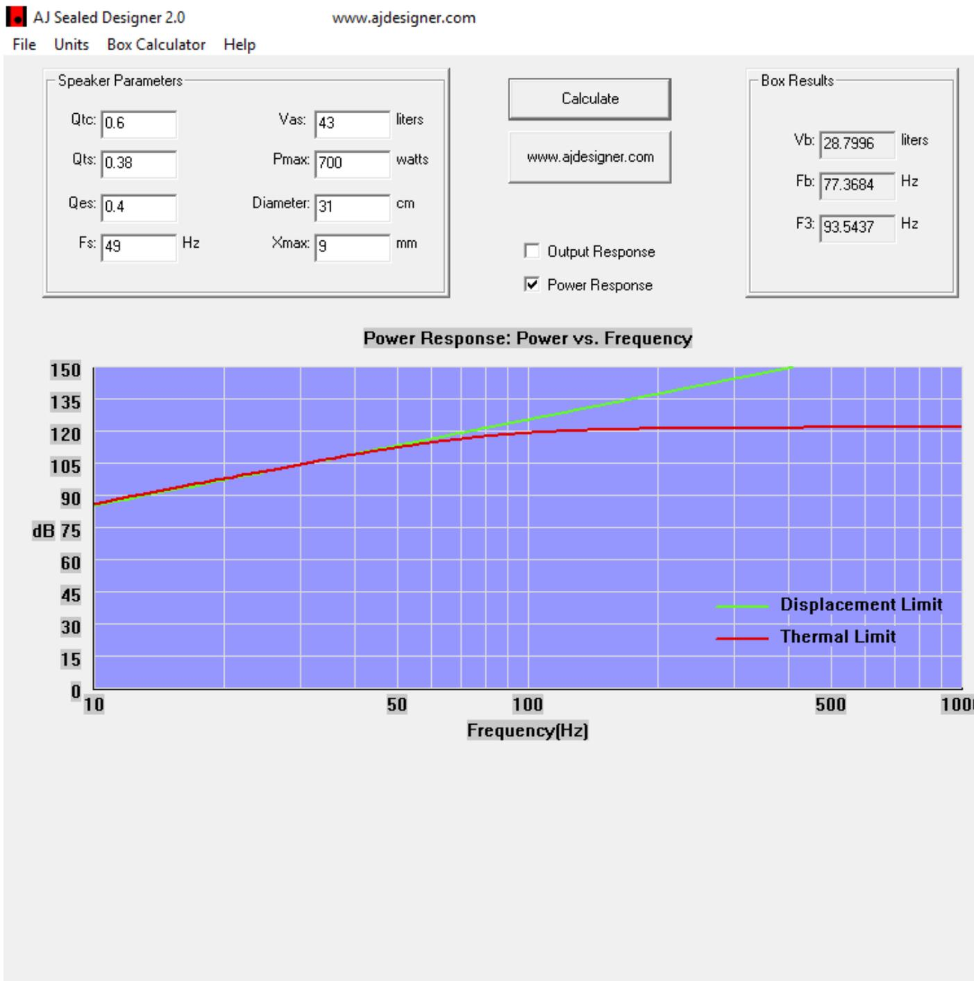
Beyma 15 P1000 V2 with 700 watts (rated at 1,000 watts AES) V2 in 38 litres sealed
