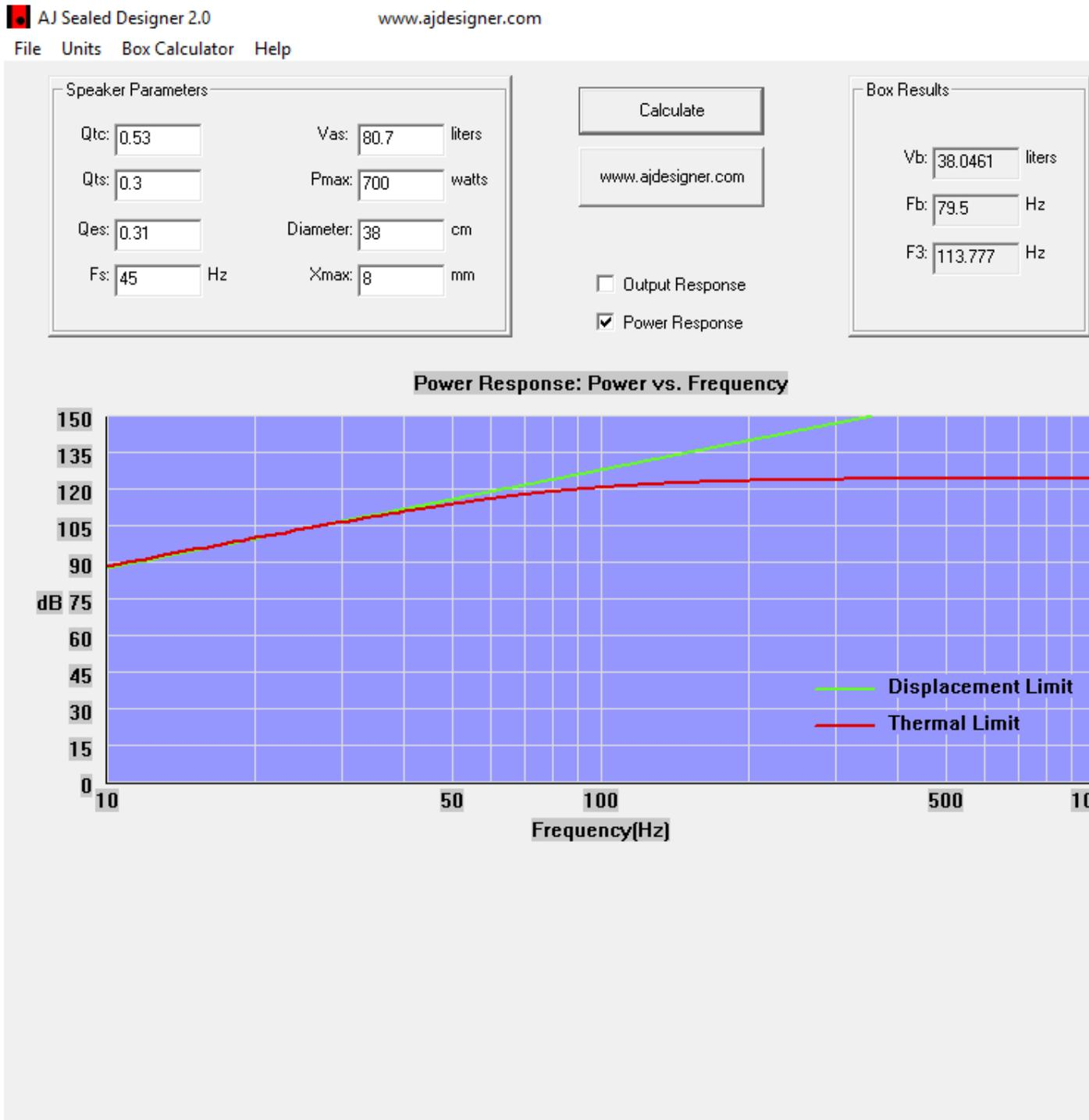
Included for fun... If you have space for a 5 cubic foot box....Beyma 21 LEX 1600 Nd in sealed 125 litres (5 cubic ft) with **500 watts (1,600 watts AES Max power!)** = 105dB @ 20 Hz with 7mm travel (13mm Xmax!)
