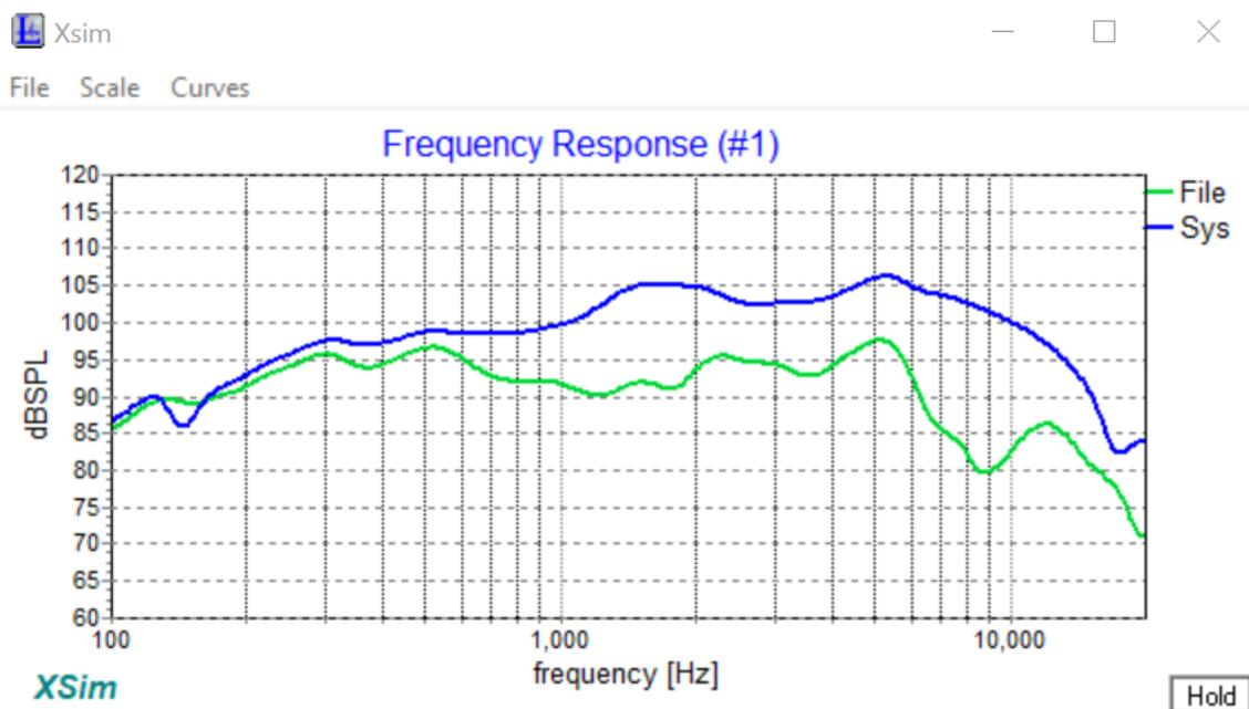
9. "Tune" the woofer driver by adjusting the delay until the curves come close together.
