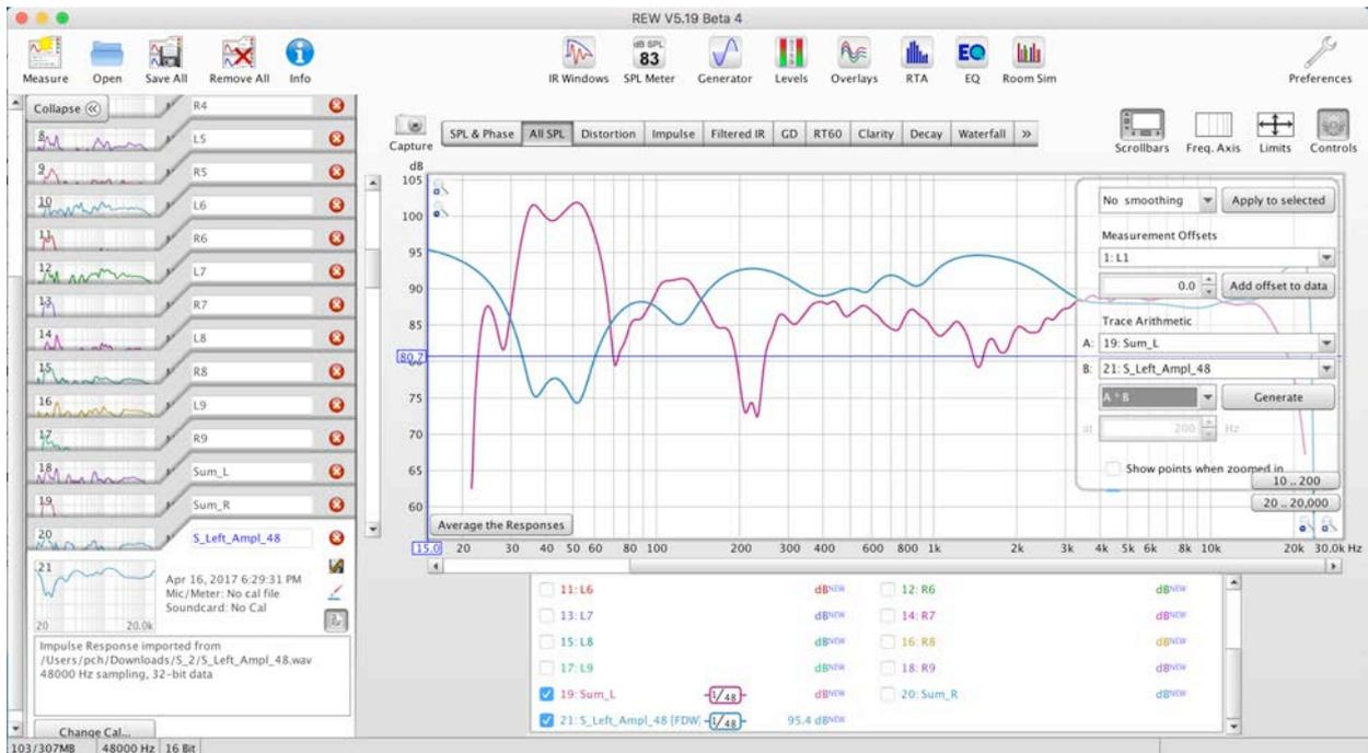
At this stage, you have generated the amplitude correction impulse and applied it to the averaged measurement. The result is an amplitude corrected measurement, which will be used to generate the phase correction.
