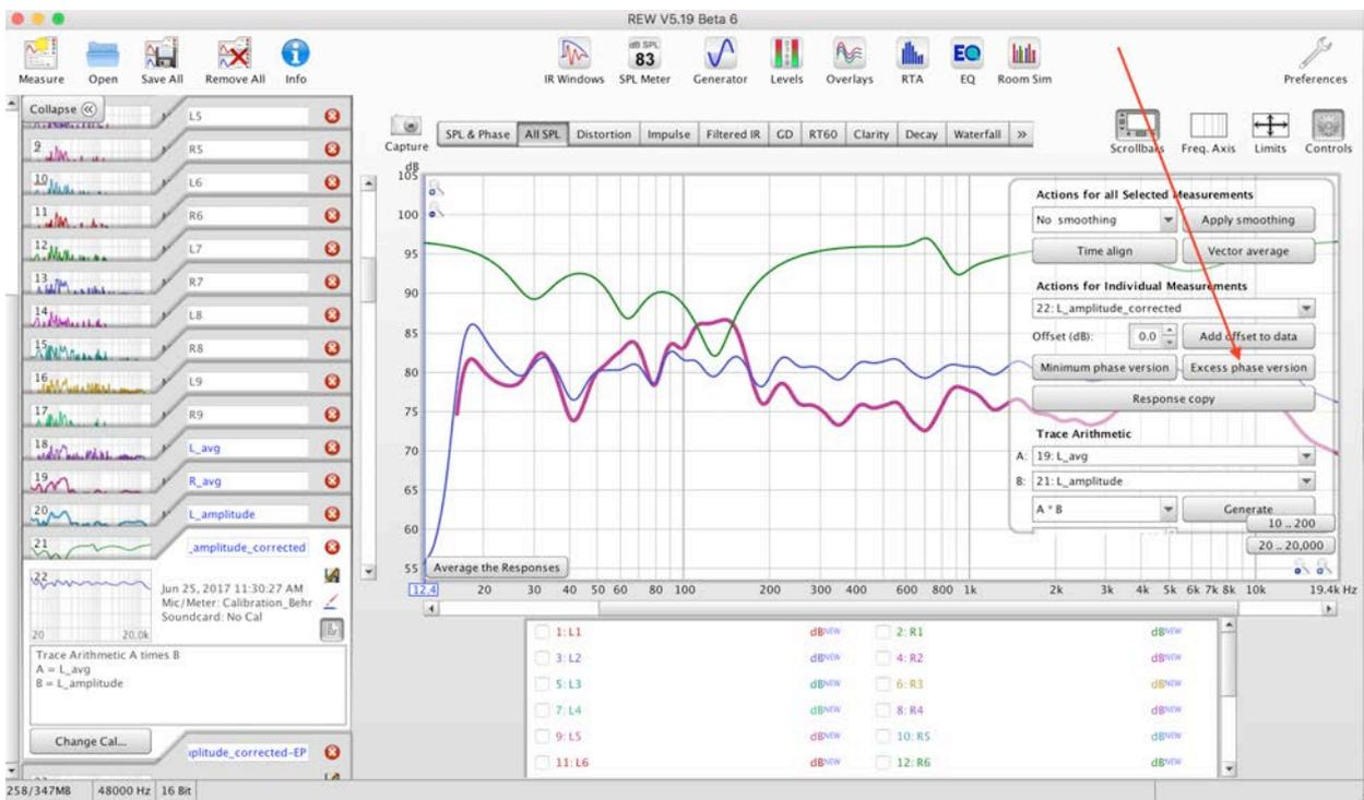
The excess phase, which has been generated, can now be exported as .txt to rePhase, where it will serve to make the time domain correction. The goal is, through Filters linearization and Phase EQ to have a phase curve close to flat at zero.
