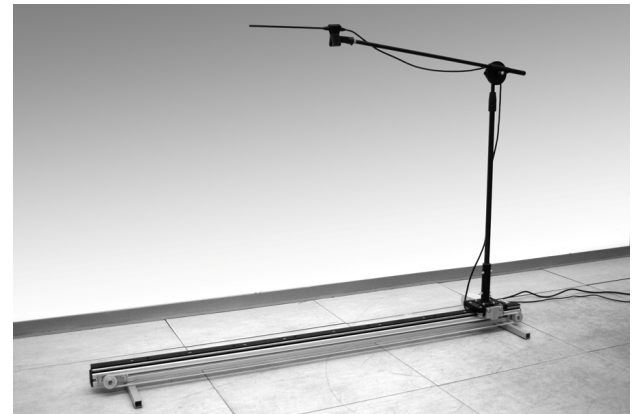
Fig. 4. Measurement microphone mounted on the linear slide
