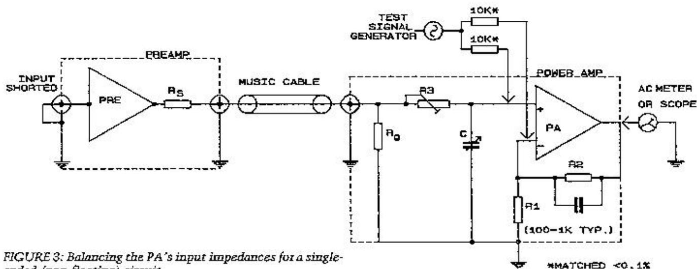
FIGURE 3: Balancing the PA's input impedances for a single-ended (non-floating) circuit.
