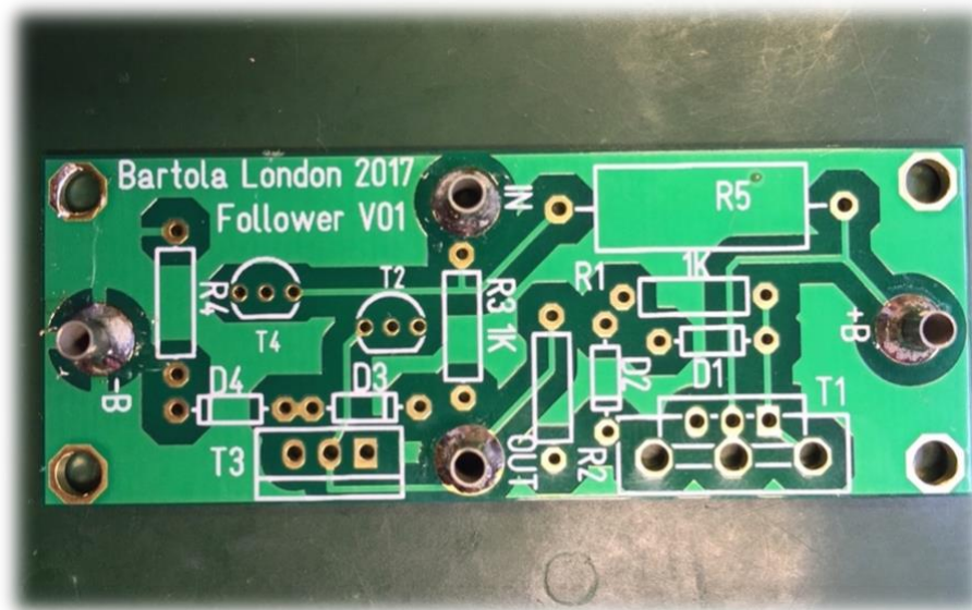
Figure 6-Step 1: solder the PCB 2mm sockets
