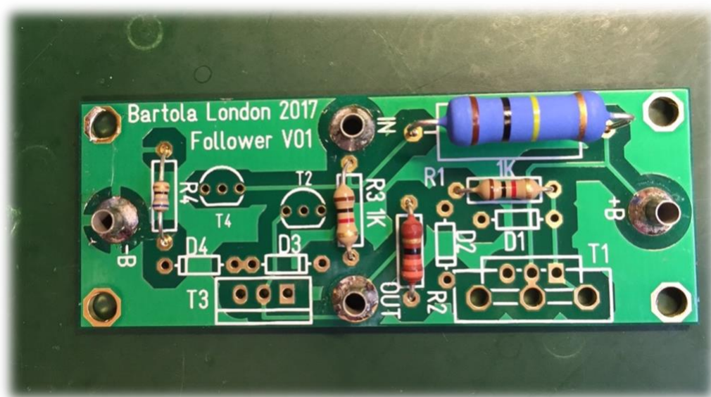
Figure 7-Step 2: solder the resistors
