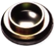
B&W has pioneered the use of hollow pole magnets to minimise back reflections behind the dome. The magnets are made from neodymium, iron and boron and are extremely powerful for their size.
