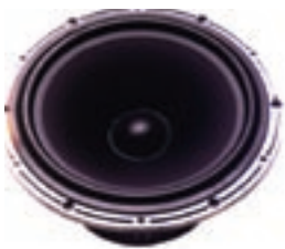
B&W's patented method of using Kevlar® for loudspeaker cones, left, has been a major factor in reducing unwanted standing waves in the diaphragm. Kevlar® was created by DuPont as a material for bullet-proof vests. B&W has made it one of the best-sounding materials for hi-fi speaker cones.
