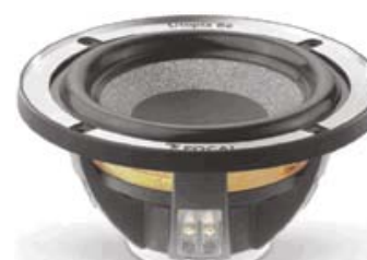
PHOTO 2: Focal 325mm woofer with sandwich type glass fiber-polymer resin/Rohacell/glass fiber-polymer resin composite "W" cone.
