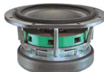
PHOTO 1: B&W 250mm woofer with TEPEX sandwich type Carbon Fiber-TPU/8mm Rohacell 31LS/Carbon Fiber-TPU composite cone.
