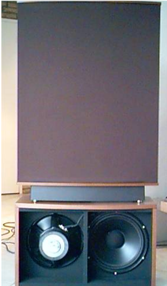
Fig 1. This sub is driven by a Quad 405. Speakers are in series. The ESL-63 is driven by Marc Levinson No 23. The ESL's are still original after more than 30 years. They are often driven up to 50Volts top to top
