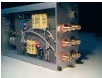
Fig. 2 The electronic crossover and correction unit.
