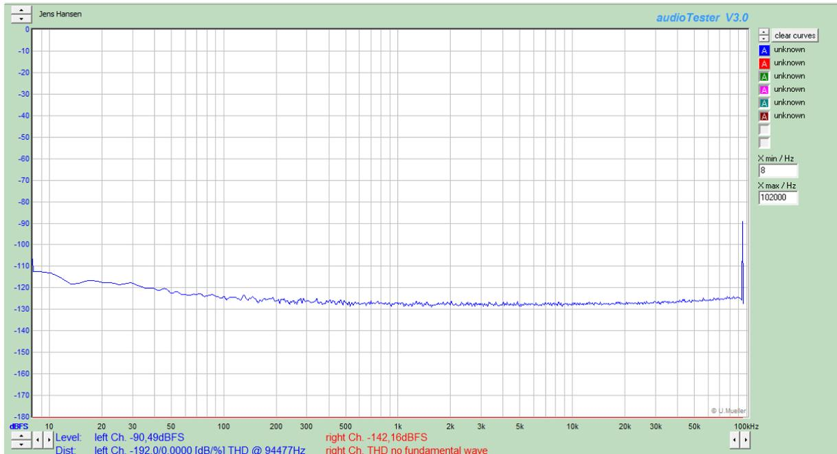
Noise over a 20kHz bandwidth = -90.49dBFS on the input. This corresponds to a level of -120.48dBFS on the generator = 9.5uVrms.
