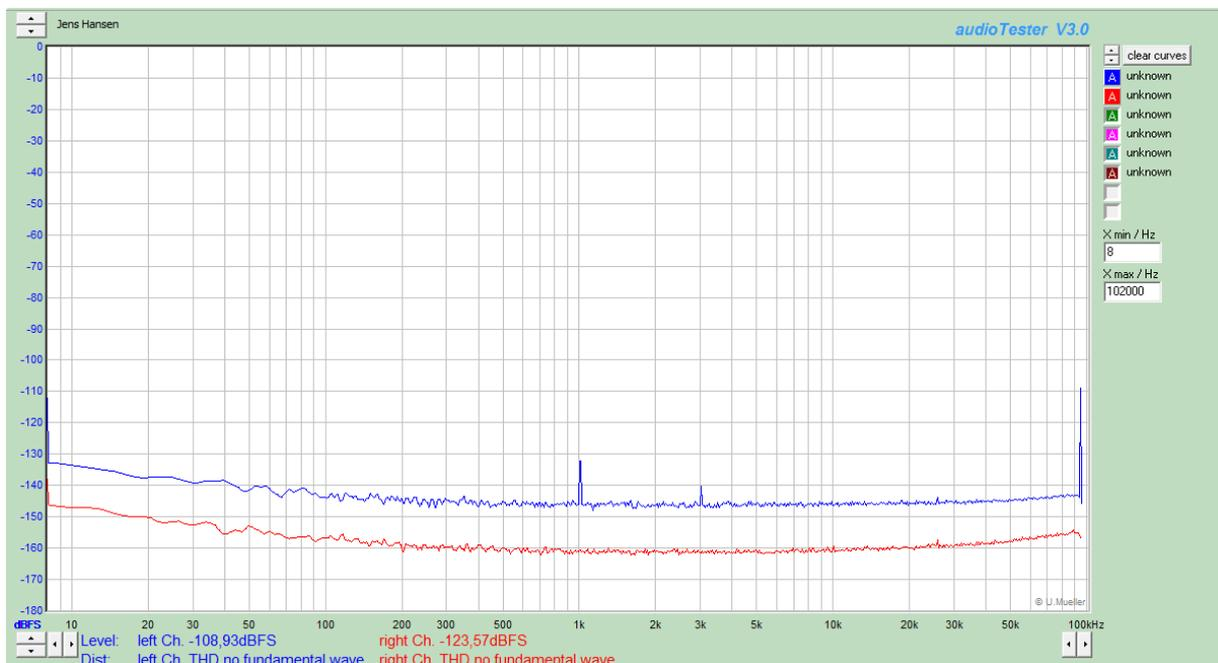
Noise over a 20kHz bandwidth = -108.93dBFS on the input. The measurement without any signal showed -108.98dBFS, so the result has not really changed. Verifying that the DAC does not "cheat" in the noise measurements.
