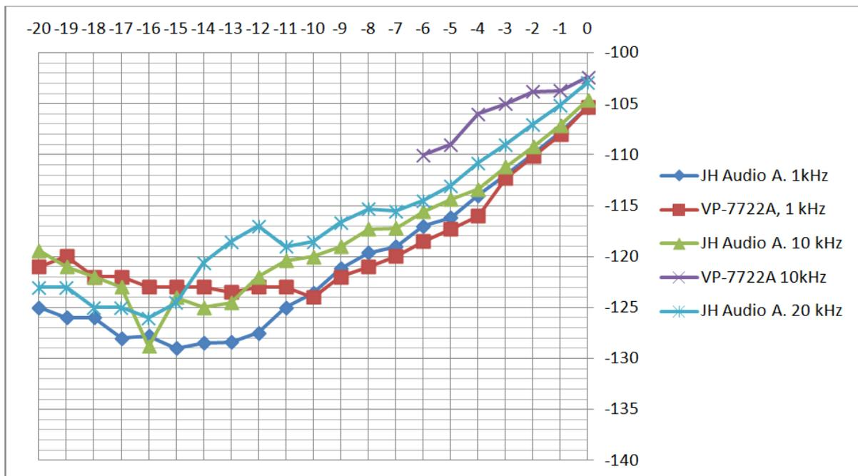
Generator distortion with AK4490. 151024. X-axis = dBFS, Y-axis = THD in dB.
