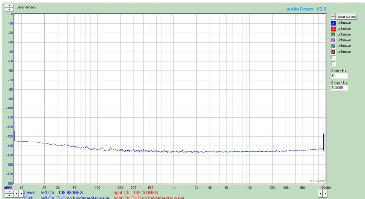
Noise over a 20kHz bandwidth = -108.98dBFS on the input. This corresponds to a level of -118.98dBFS on the generator = 3.6uVrms.
