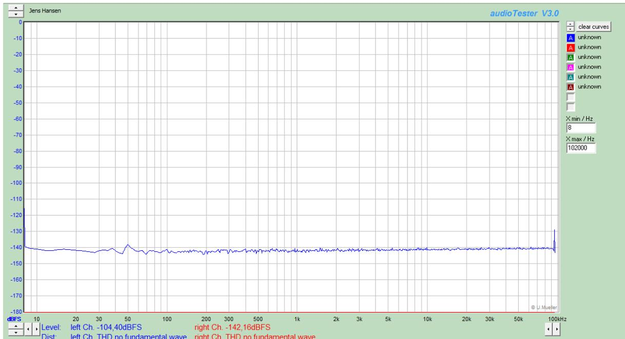
Noise over a 20kHz bandwidth = -104.40dBFS on the input. This corresponds to a level of -128.98dBFS on the generator = 0.6uVrms.
