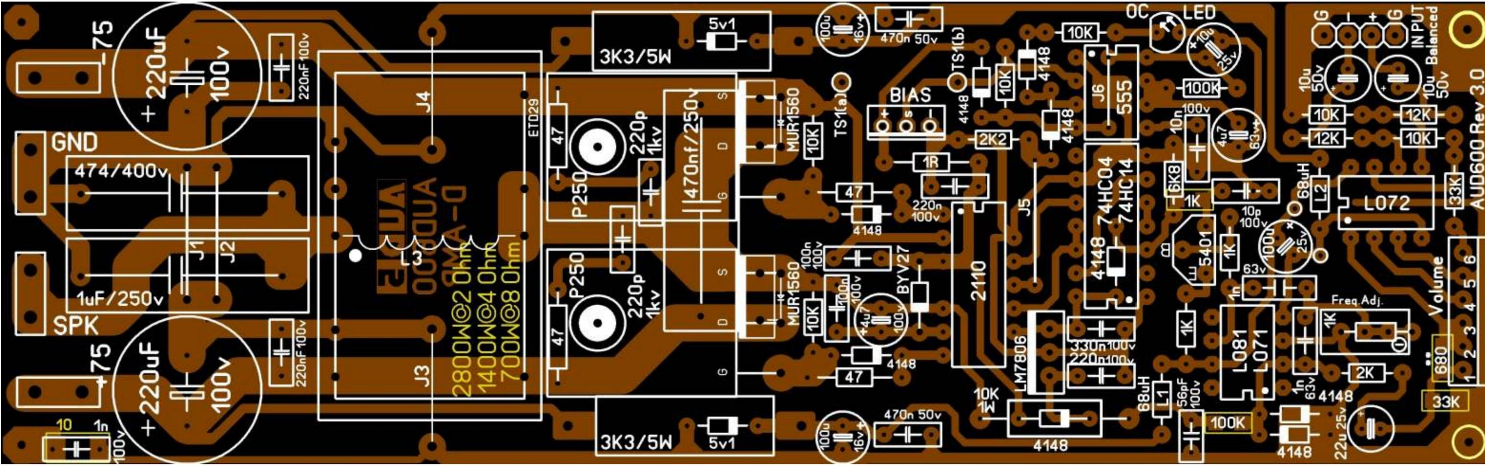
\*\* Remove Resistor 680 Ohm and connect Limiter/EQ/Tone board in between Pin 1 & Pin 2.
