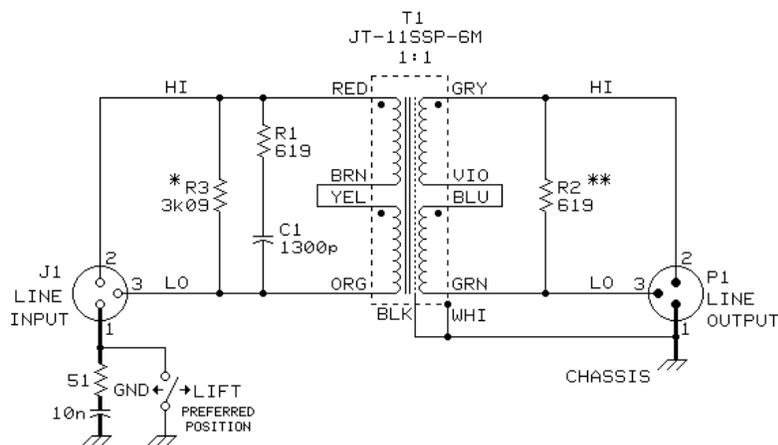
\* INPUT IMPEDANCE IS 743 OHMS WITHOUT R3. IF 600 OHM INPUT IMPEDANCE IS REQUIRED, USE R3 AS SHOWN.
