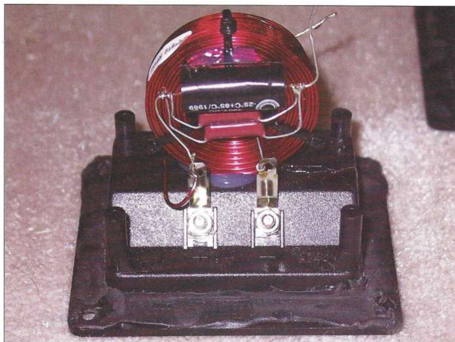
PHOTO 3: The assembled crossover network.
