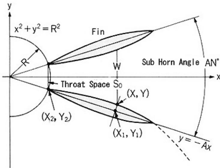
This is the top view of single horn cell or a sub horn. Each horn cell is to be aligned with angle AN. The center horn cell starts from X2. And each throat of the horn cell is located on circle R. It is easy to understand the factors of horn space expansion horizontally. The contribution factors are the radial expansion and the thickness of the fins up until the end of the fin area.
