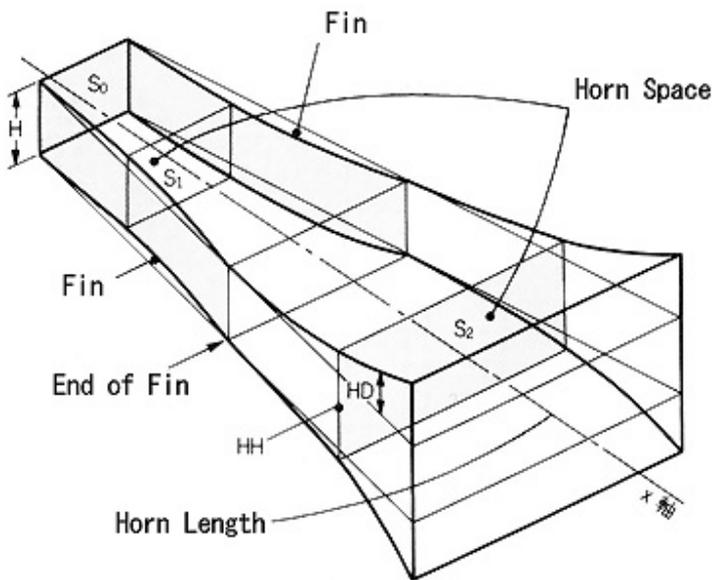
Left fig. shows a model of single horn cell. In this case, above horn consists of five small horn cells. A horn cell consists of two horn space expansion mode, S1 and S2.
