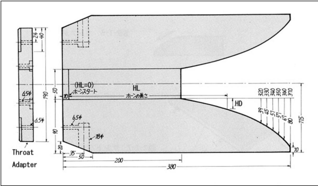
This is the side view of the horn. The thickness of the wood material at the mouth location keep 1cm to minimize vibration. The throat of the horn cell is located 1cm inside of the horn throat. This came from the drawing of the top view.
