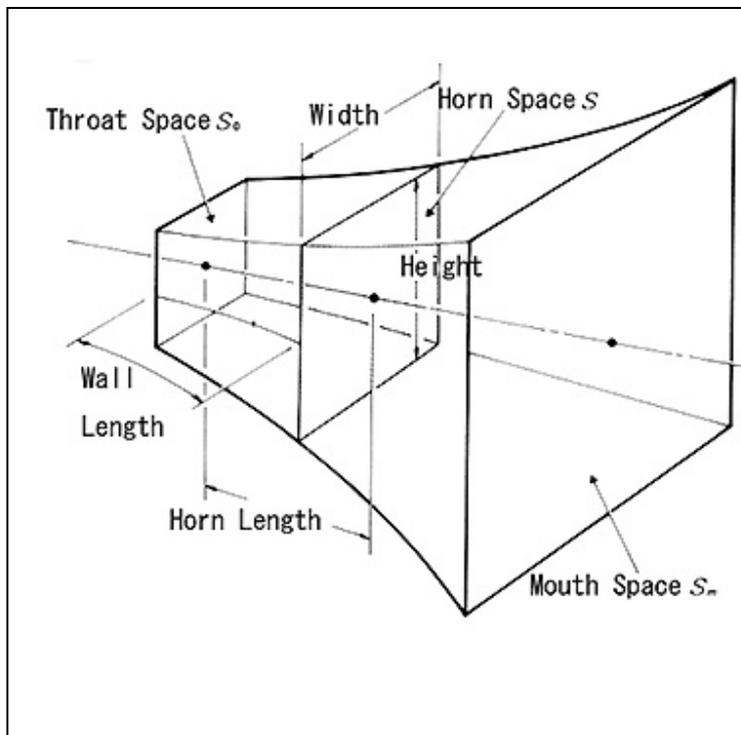
The horn expands its horn space ( $S$ ) from the throat position ( $S_0$ ) to the mouth ( $S_m$ ). "How it expands" depends upon the equation which is so called horn type. Which includes the "Exponential", "Hyperbolic", "Cone" and "Tractric". Since the Tractric horn expands its horn space up until the infinite baffle, its horn length is limited. Other horns have unlimited horn length. Therefore, we cut the horn length intentionally because we can not make it.
