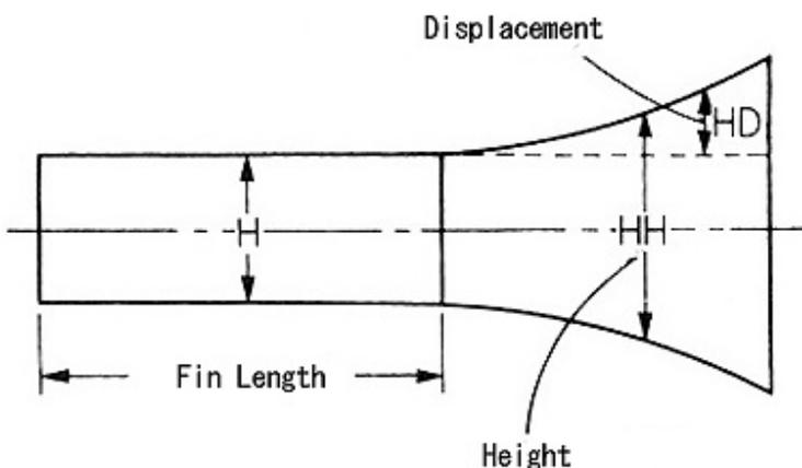
This is the side view of the horn cell or the sub horn. It is easy to understand the factors of horn space expansion vertically. In the fin area, the contribution to the horn space is horizontal only because the height (H) stays the same. After the fin ended, displacement of the horn height (HD) complements the radial expansion to keep S2.
