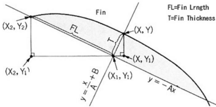
This is the cross section of the fin. On this chart, "T" means half of the fin thickness. Therefore, T\*2 is the thickness.
