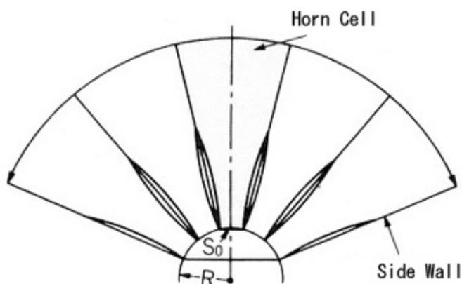
Now we can design the horn system. The reason why the A-290 has several fins inside is as follows. Without fins the high frequency sound over 8KHz concentrates in the center of the horn. Therefore, the separator is important to have flat frequency response to provide wider service area in front of the Horn. Just thin separators will create some problems. Therefore, the fins have to be reasonably robust.
