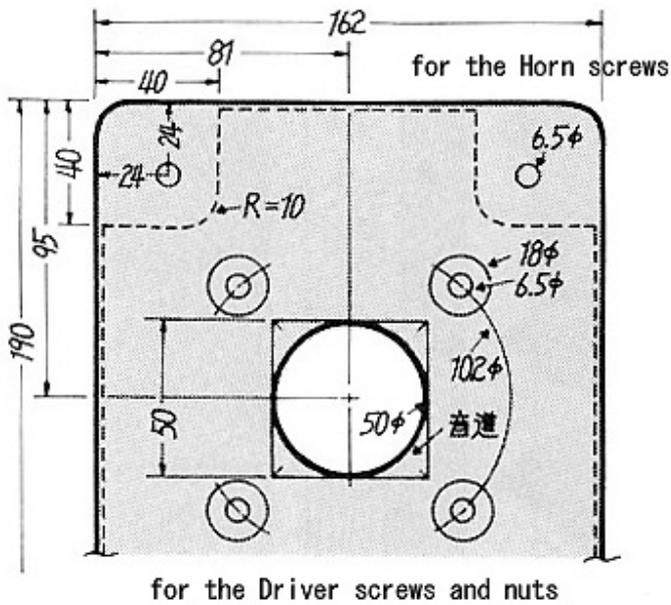
This is the drawing of the throat adapter. There are two requirements to this component.
