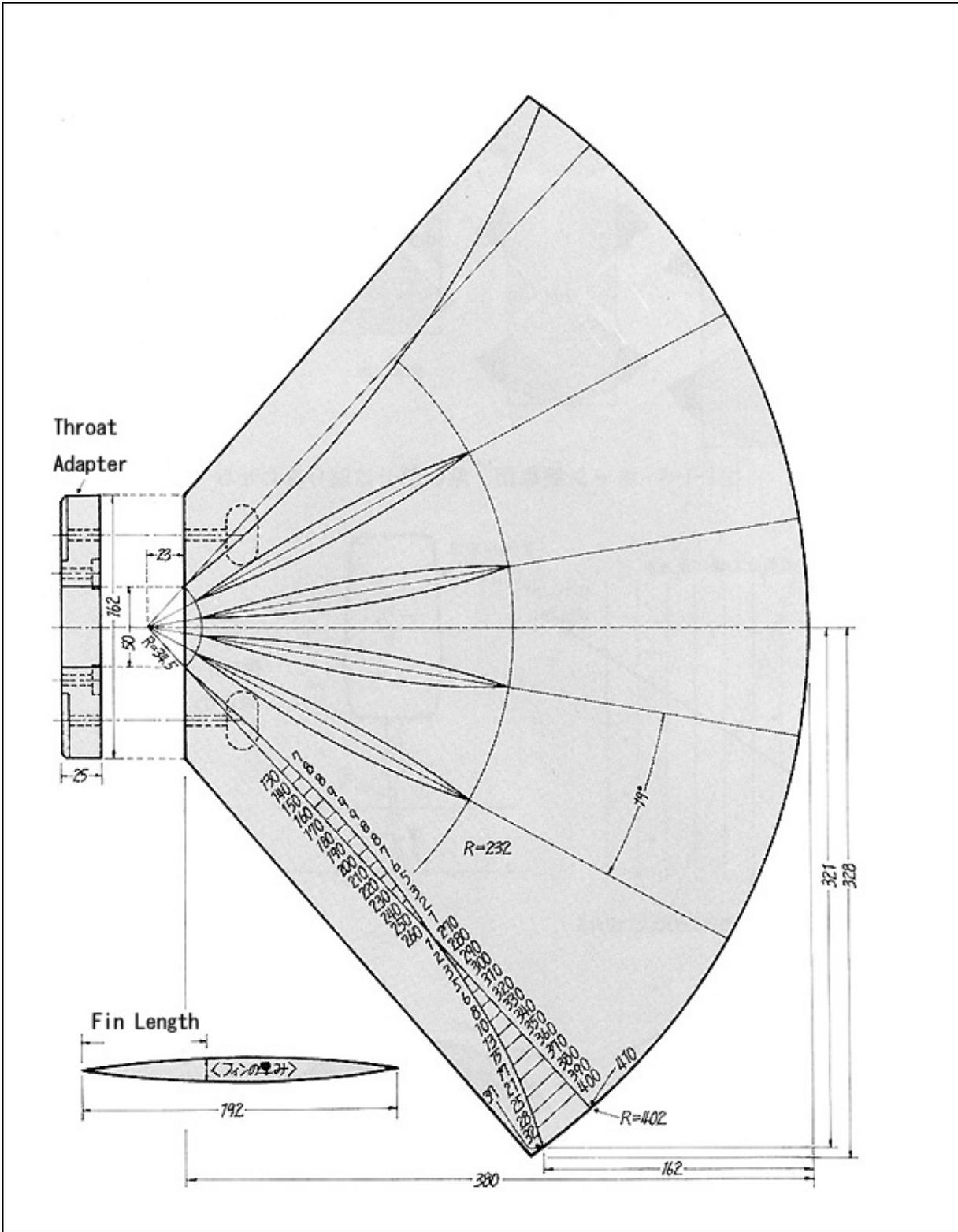
Above is the calculations. To do this, I cared about available size of wood materials, possibility of process, thickness of the fin, the mouth contour, side wall contour, angle of the horn, and other factors.
