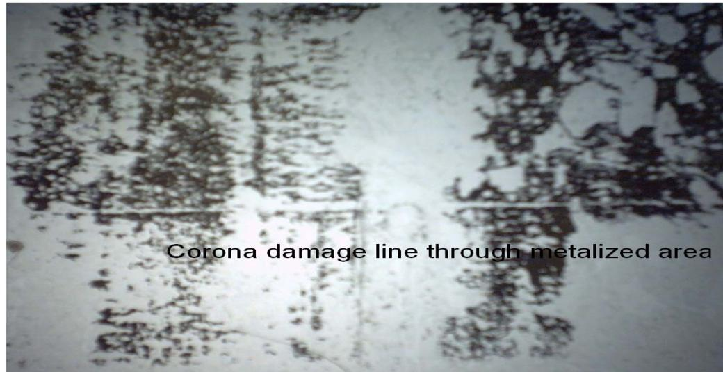
Corona damage line through metallized area
