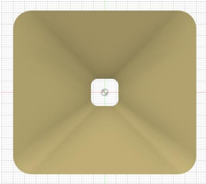
Next step is to loft surfaces between the outside and waveguide profiles to fill the gaps.
