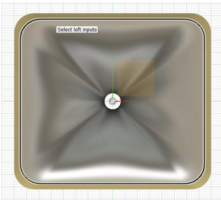
Execute the command and the surface will be created, then flip the model over to do the same on the bottom
