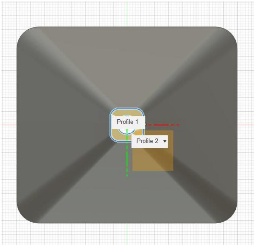
The use the stitch command to join four surfaces together, flip the model around so you can select the bottom and top lofts, the inside and outside waveguide surfaces then run the command.
