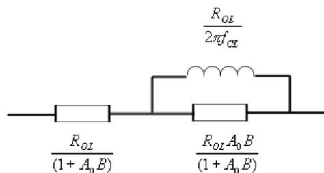
And the equivalent closed loop output impedance may be represented as a series resistor equal to the DC output resistance divided by the loop gain, and a parallel combination of a resistor nearly equal to the DC output resistance and an inductor whose value is also the DC output resistance but divided by the closed loop bandwidth.
