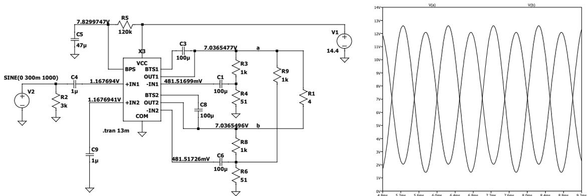
The resistor  $R_9$  and  $R_8$  provide zero point for the output. The input transistor of the following amplifier is trying to keep the voltage on the emitter constant, compensating the output of the  $\{b\}$  amplifier in opposite direction of the output of the  $\{a\}$  amplifier.
