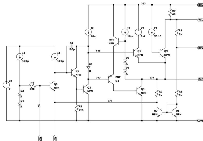
The circuit of the TDA2005 has additional input for the bootstrap (BTS) and for the bias offset (BPS). The classical bootstrap circuit requires resistor to the supply rail. The measured value between BTS pin and VCC pin is  $R_9=68\Omega$ .
