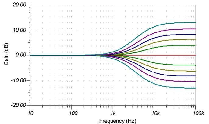
By varying R4 we can give the user control over the corner frequencies. In the next figure, the potentiometer is swept from 1k to 100k in eight log steps.
