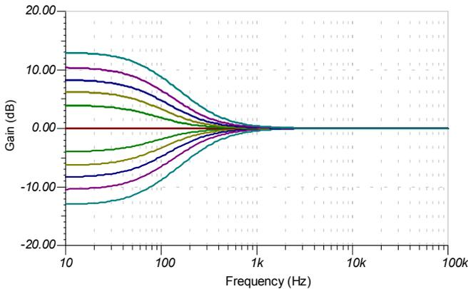
We can make a more versatile tone control if we replace R4 with another potentiometer wired as a variable resistor.
