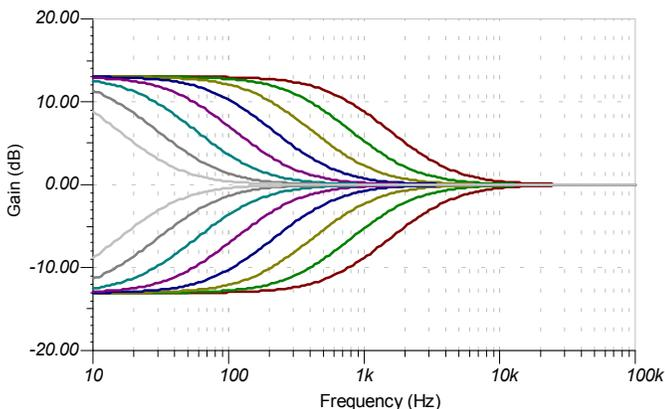
Sweeping this potentiometer from 1k to 100k in eight log steps will vary the corner frequencies while maintaining the maximum boost or cut.
