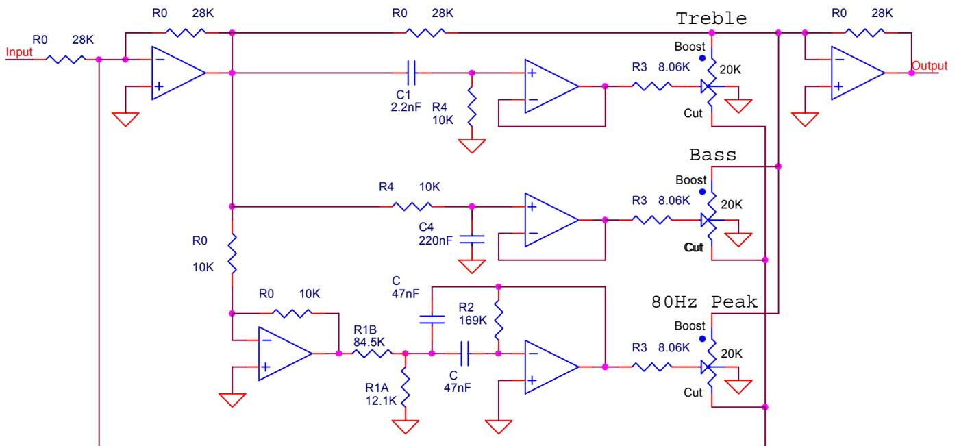
**Schematic showing bass, treble, and peaking tone controls**
