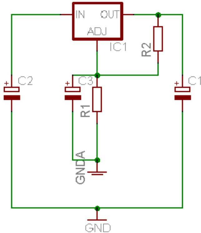
Connect GNDA as close as possible to 0V pin(s) of device being powered
