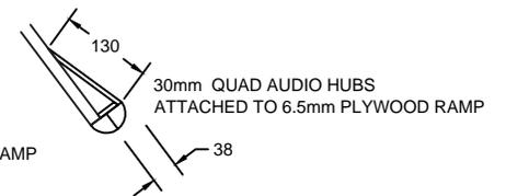
30mm QUAD AUDIO HUBS ATTACHED TO 6.5mm PLYWOOD RAMP
