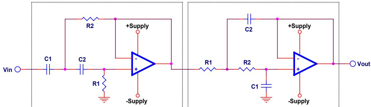
**Figure 13. Wide Band Pass Filter for  $\pm$  Supplies**
