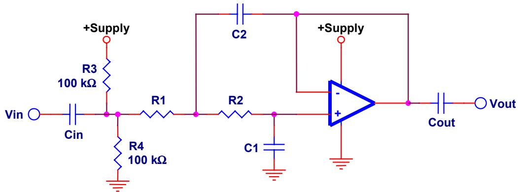
Figure 8. Low Pass Filter for a Single Supply
