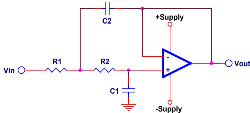
Figure 7. Low Pass Filter for  $\pm$  Supplies
