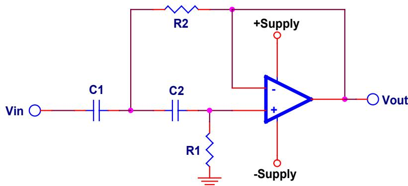
**Figure 9. High Pass Filter for  $\pm$  Supplies**
