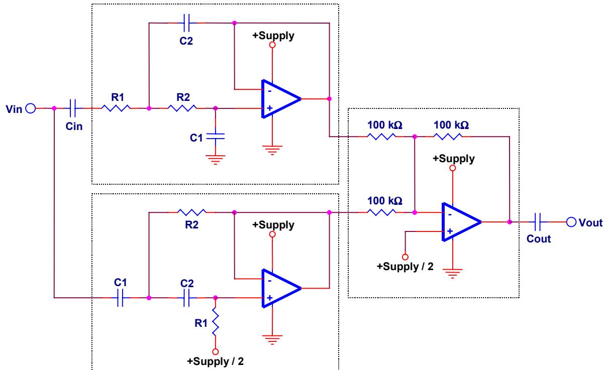
**Figure 18. Band Reject Filter for a Single Supply**
