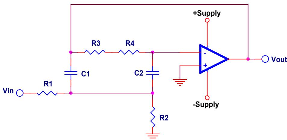
Figure 11. Narrow Band Pass Filter for  $\pm$  Supplies
