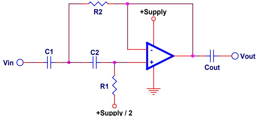
**Figure 10. High Pass Filter for a Single Supply**
