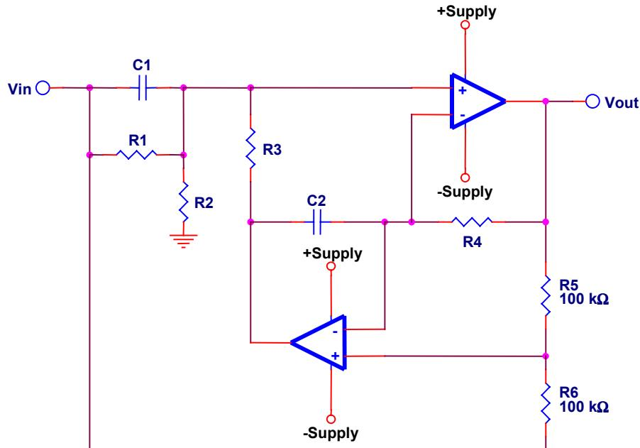
Figure 15. Narrow Band Pass Filter for  $\pm$  Supplies
