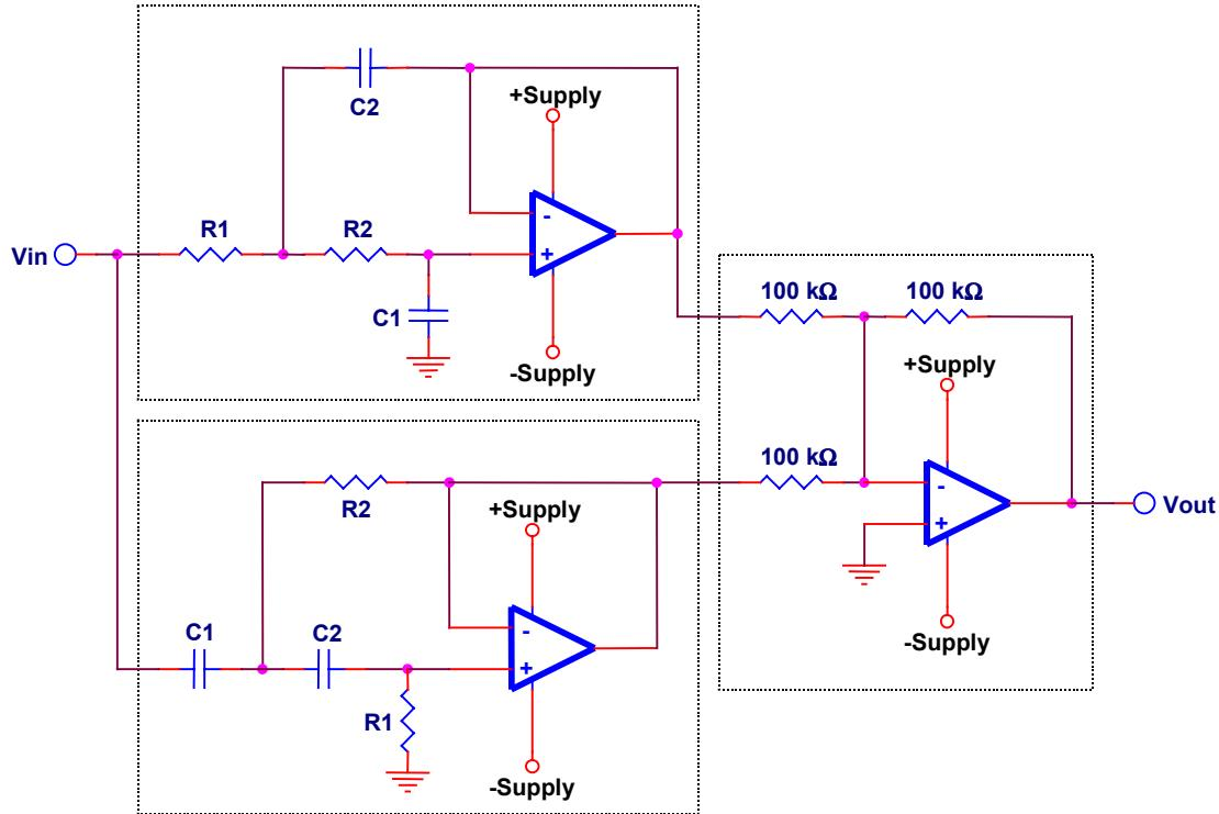
**Figure 17. Band Reject Filter for  $\pm$  Supplies**
