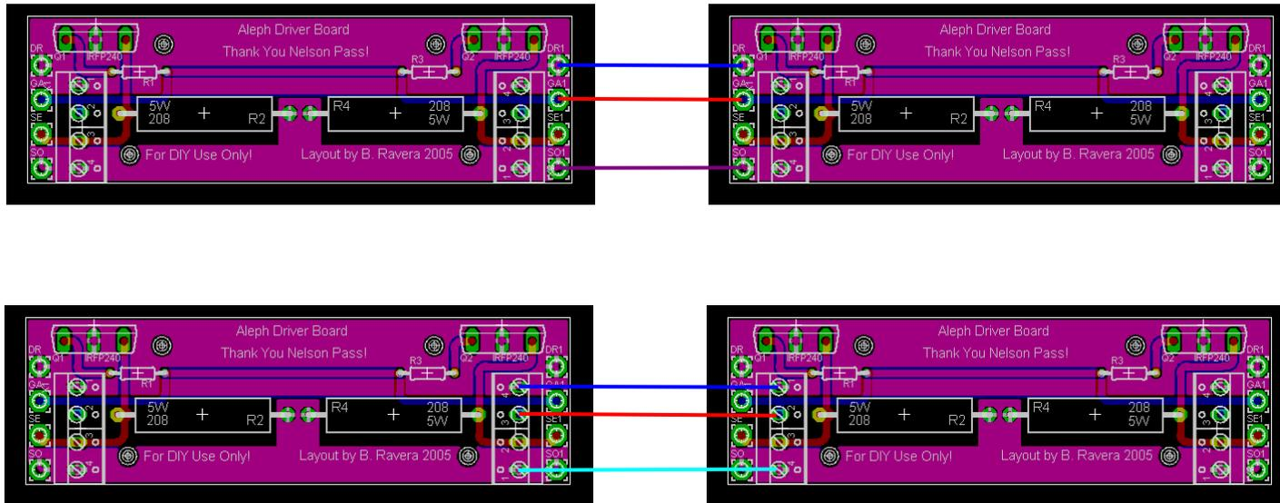
When chaining two or more boards, the SENSE contacts (SE...) MUST NOT be connected
