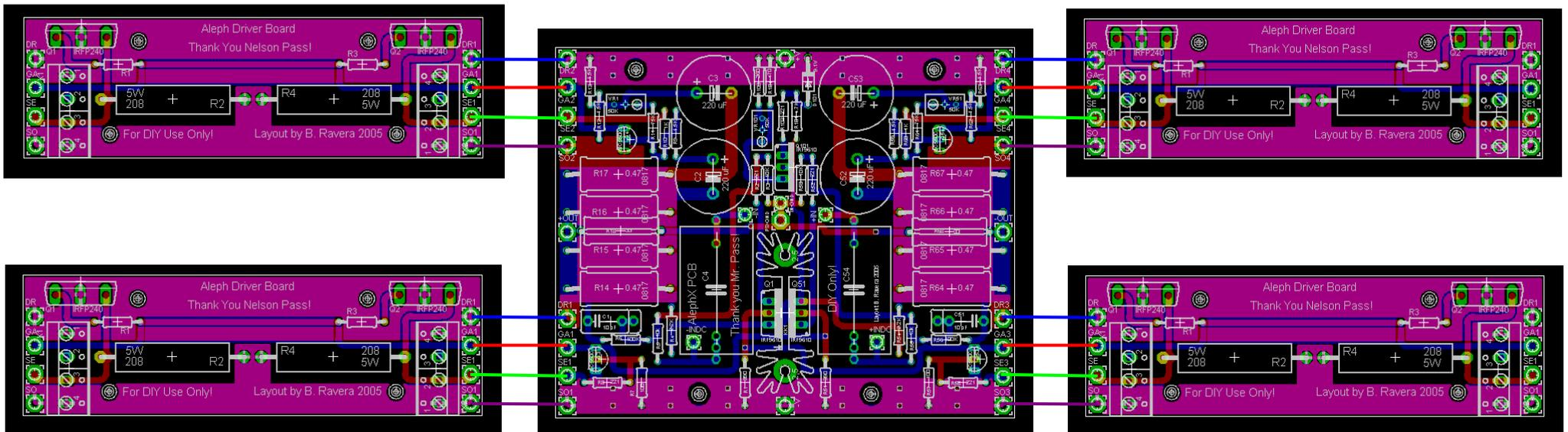
Note: the driver boards can be connected also via the screw connectors X1 and X2
