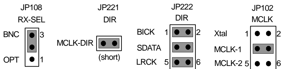
Figure 3. Jumper Pin Settings with DIR
