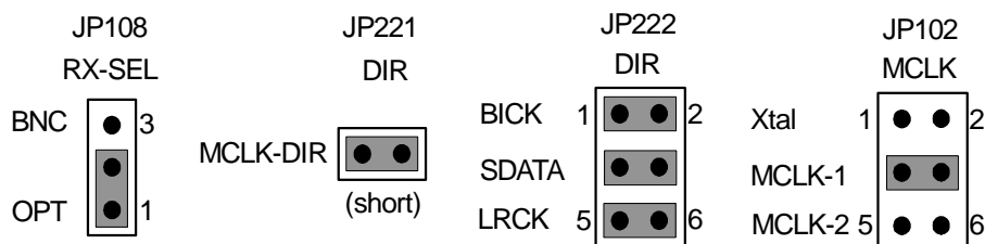
Figure 4. Jumper Pin Settings with DIR
