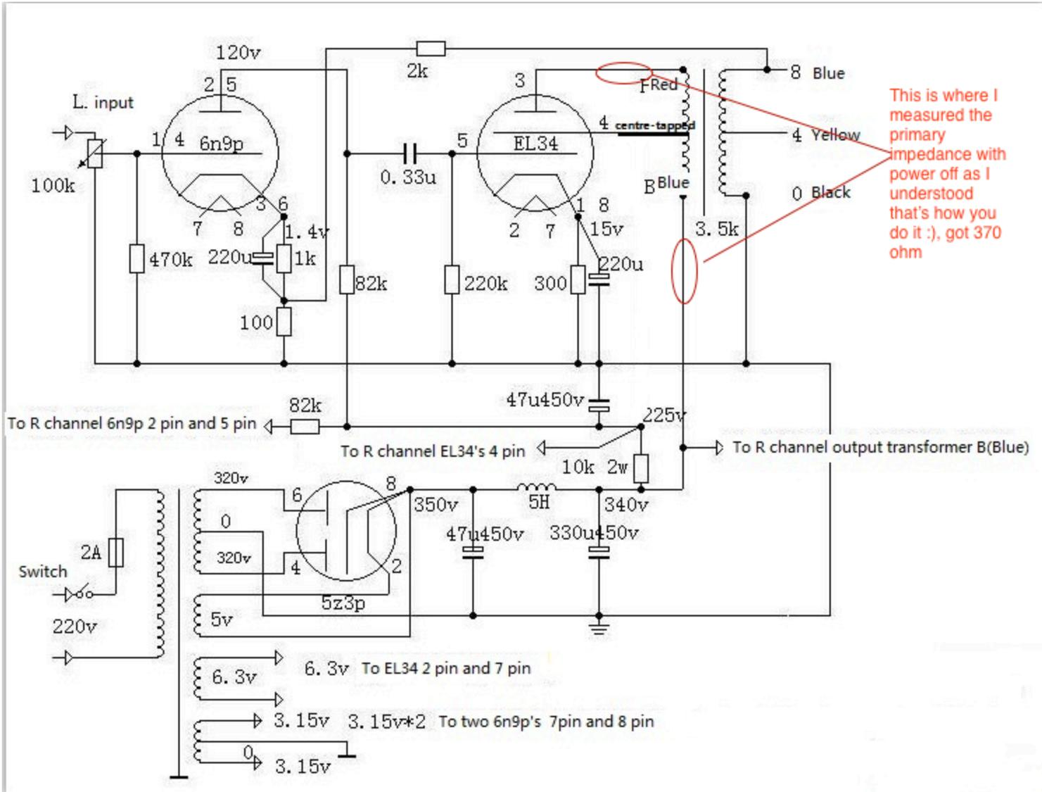
Note: if power transformer have just 1 group 6.3v output, then two EL34 shared it else when it's have two group 6.3v outputs, then each for one el34's 2 pin and 7 pin
