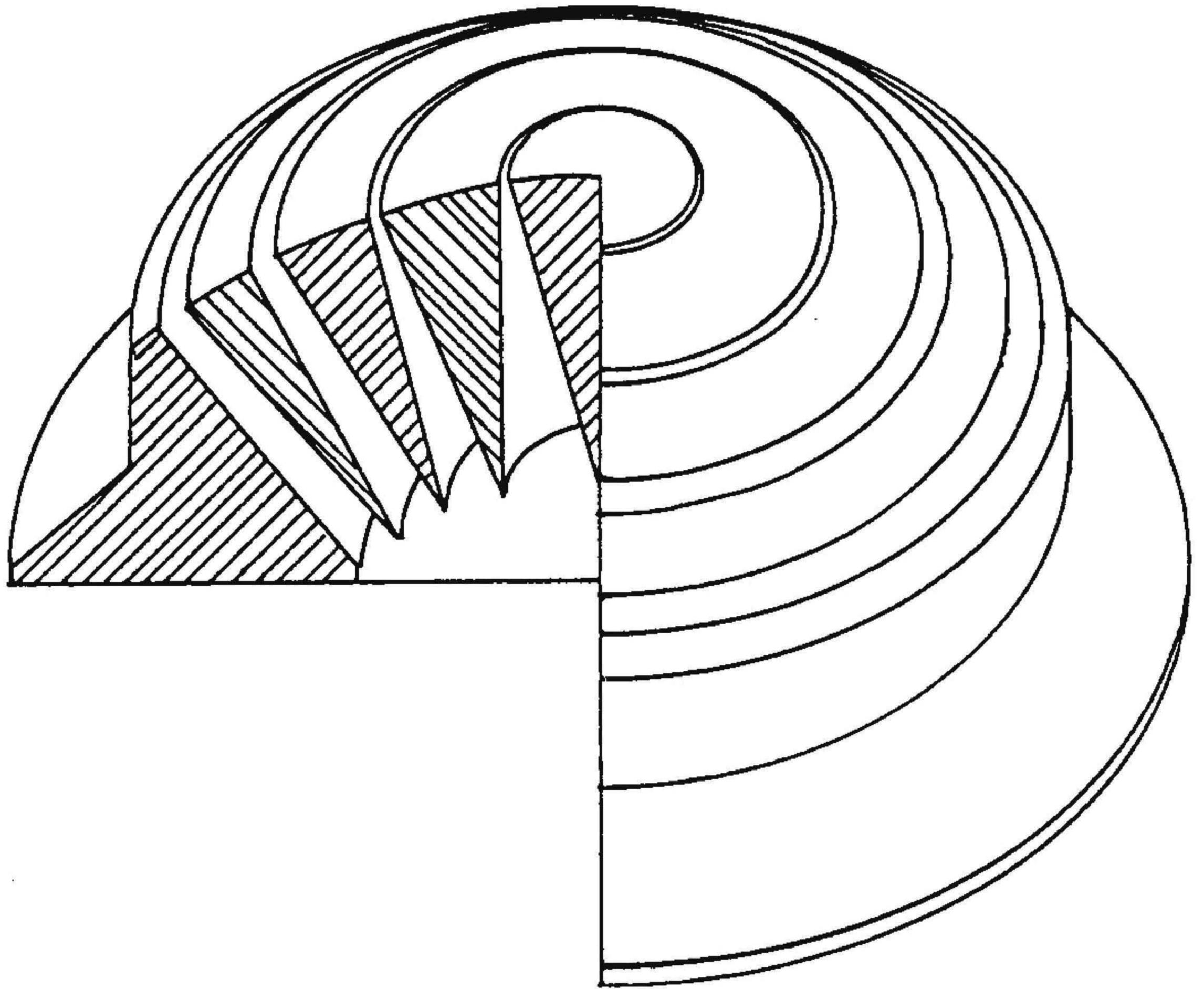
Figure 5. Concentric Ring Phasing Plug and Pole Piece - after Smith
