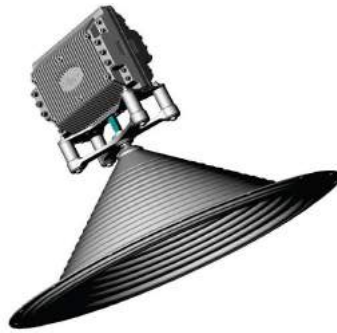
Figure 8 - A 3D drawing view of moving magnet transducer attached to a 30" cone.
