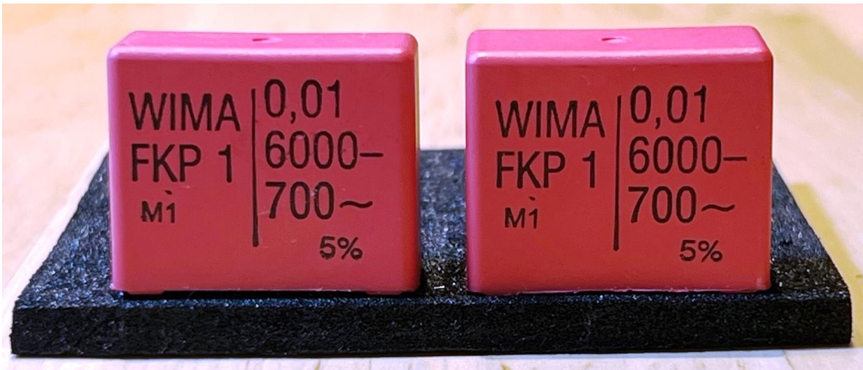
Figure 14. WIMA high-voltage capacitors, type FKP1Y021006F00JSSD
