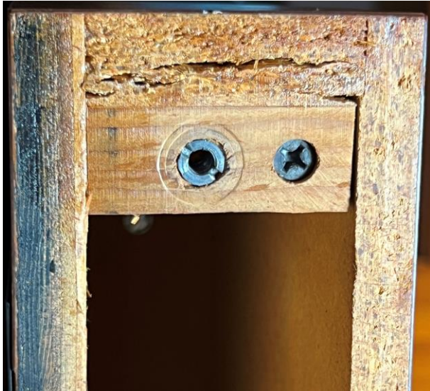
Figure 21. Underside of wooden frame base showing split in the particle board.
