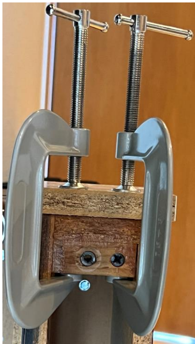
Figure 22. Clamping of wooden frame base – a spacer board helps even the c-clamp force.
