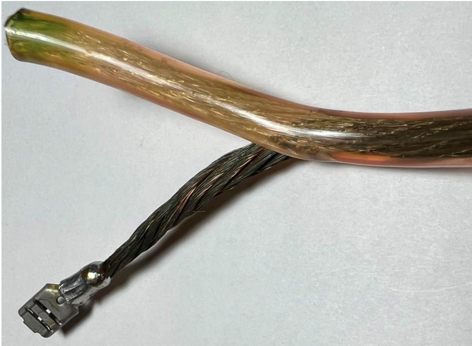
Figure 3. Discolouration in low-frequency wiring conductors – sheath pulled back for clarity.
