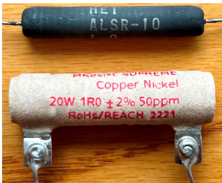
Figure 17. Original Huntington Electric 1-ohm 10W resistor ( top ), Mundorf MResist Supreme 1-ohm 20W resistor ( bottom ).
