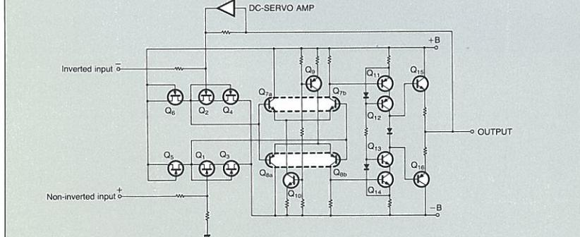
Fig. 3 Circuit diagram for the balanced input amplifier
