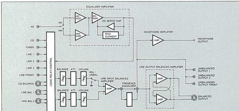
Fig. 1 Circuit block diagram of C-260 (one channel)
