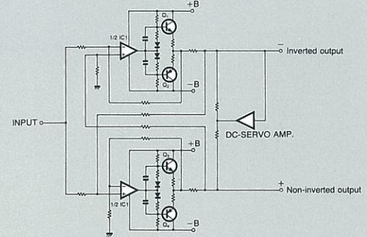
Fig. 4 Circuit diagram for the balanced output amplifier
