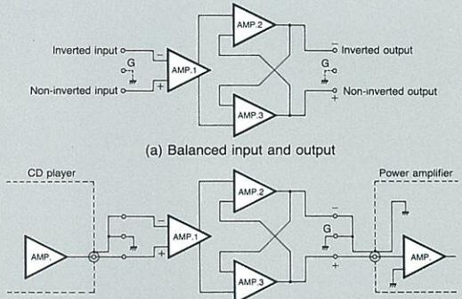
Fig. 2 Balanced line amplifier stage
