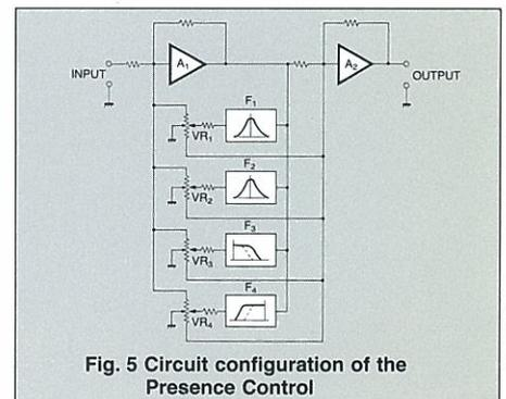
Fig. 5 Circuit configuration of the Presence Control
