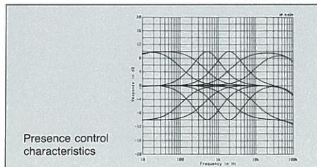
quency range are set at 500Hz and 2kHz. The 500Hz control can effect, for example, the timbre of rhythm instruments and the 2kHz control can be used to emphasize vocals or reduce traces of stringency.
