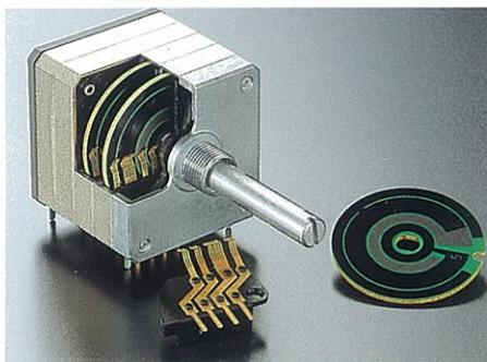
collectors that are connected directly to the external terminals. This construction has successfully reduced the number of metal joints from 5 to 3, thus greatly contributing to the improvement in sound quality. This volume control is a precision 4-ganged type, controlling the positive and negative signals of the left and right channels simultaneously. It is ganged so precisely to ensure a smooth rise in sound levels of both channels.
