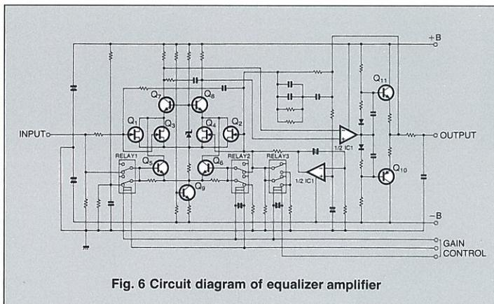
Fig. 6 Circuit diagram of equalizer amplifier
