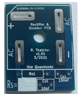
Bridge Rectifier & Snubber PCB Also: CL-60/AC cap PCB GPBC / CL60 bridge ground PCB
