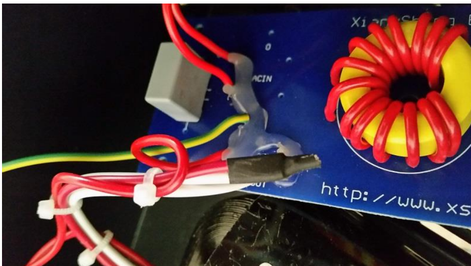
Proper Yellow/Green Ground wire fitted to PCB.
