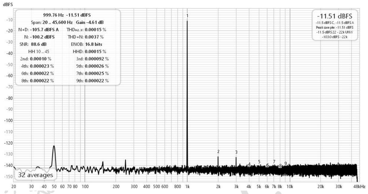
The 50Hz comes from the lab supply used in the measurements.
