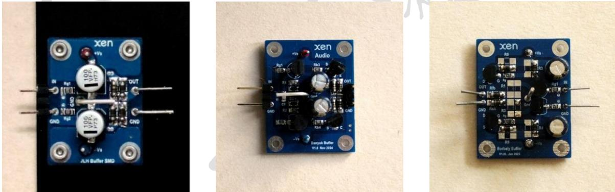
Earlier in the Le Monstre Preamp thread, we posted schematics and spice files for 3 different line level buffers, which all have JFET inputs and use 4 complementary transistors in total. For our curiosity, we have now built and measured them all, as shown above.
