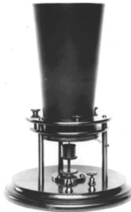
Bell's original liquid transmitter microphone
